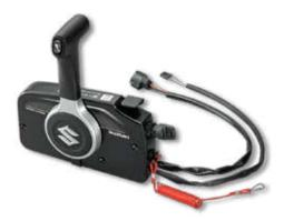
SIDE-MOUNT REMOTE CONTROL BOX for Single-Engine
